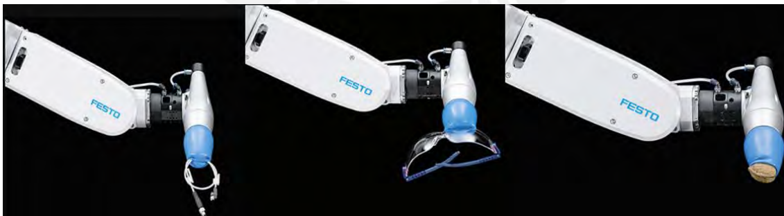
Fig. 1.17: Gripper fitting capability, examples of gripper’s form adaptability. [27]
