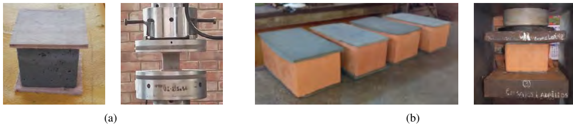
Fig. 1. Specimens and experimental set-up for masonry materials: (a) compressive test on joint mortar; (b) compressive test on brick.
