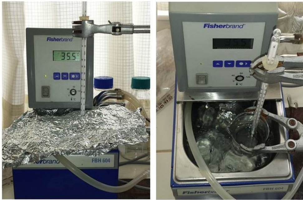
Figure A.11: Measurement setup for determination of transition temperature T_{tr}
