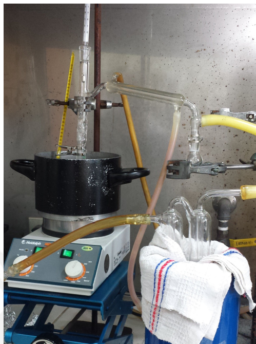
Figure A.1: Purification of 2-methoxycarbonylethyl-2-oxazoline (FOxa) by vacuum assisted distillation
