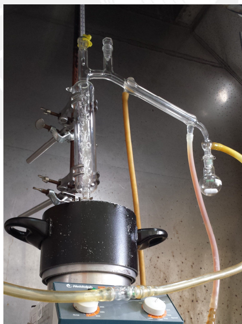
Figure A.2: Purification of 2-methyl-2-oxazoline (MeOxa) by distillation
