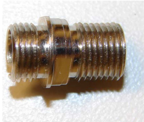
Figura 3-3: Adaptadores FC/PC o FC/APC Fuente: [Alcatel Lucent Technologies. SAC Network Cable]
