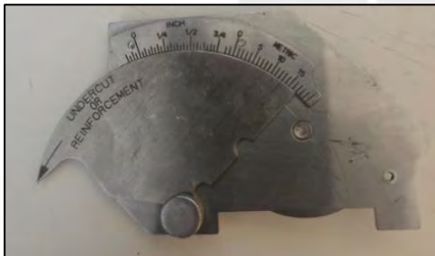
Figura 38. Bridge Cam gauge
