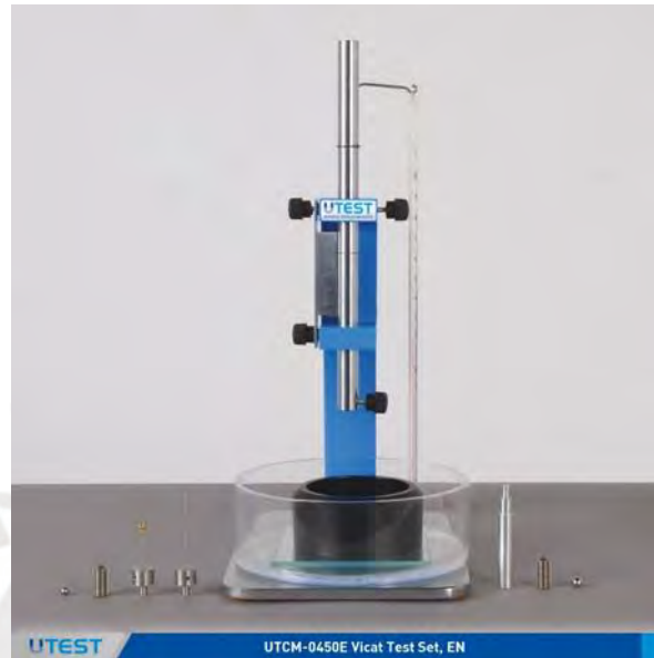
Figure 3.4. Vicat equipment of the UTEST brand was very similar to the one used for the tests in this section (UTEST, 2023).
