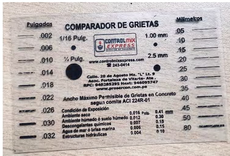
Figure 3.6. This fissurometer was used to measure crack widths.
