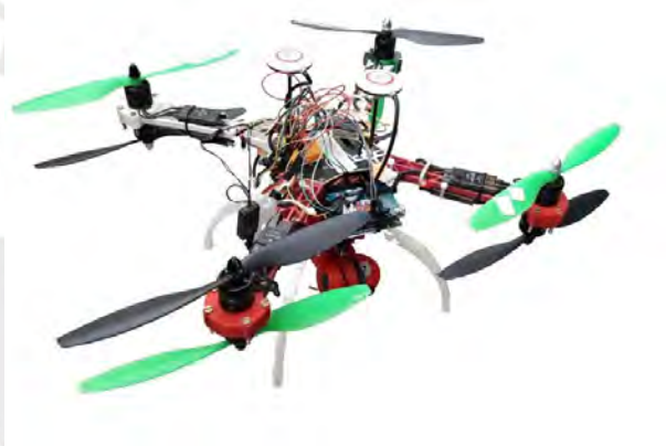
Figure 1.1: Typical quadrotor that is used for testbed of control algorithms [9].
