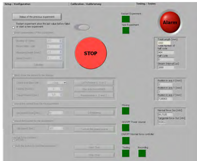
Figure 2.15: The Testing guides the user in setting the tribological and electrical parameters for the test. it then assists the user in establishing the initial normal force, making contact with the sample, setting the current, starting the test, recording the test and stopping the test upon user request.
