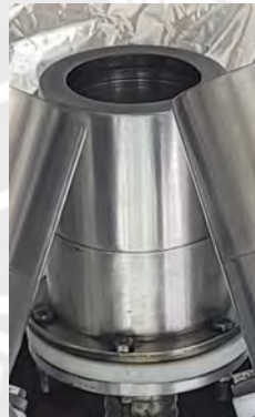
Figure 2.9: Image of a self-made magnetron manufactured in the MatER PUCP laboratory.
