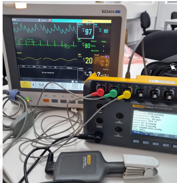
Figure 2.10: Setup for storing ECG generated by the ProSim 8 to the Monitor EDAN iM70
