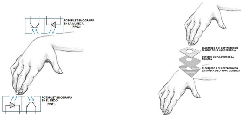
Figure 2.6: Lead 1 ECG in a wearable [8]
