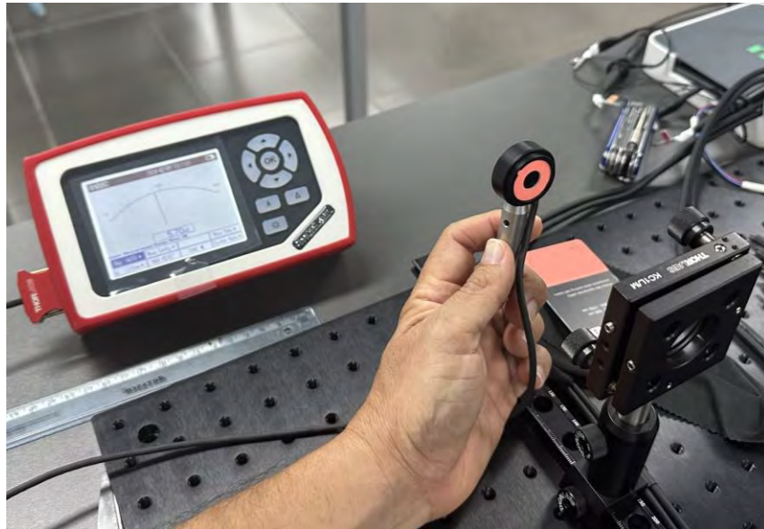
Figure 4.19: An optical power meter, Thorlabs PM100D, was placed at the Sample arm. The value obtained was 5.33 mW, one third of the allowed power, according to the International Electrotechnical Commission (IEC) recommendation.
