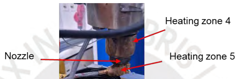
Figure 3.14. Nozzle and heating zones of customized screw extruder.
