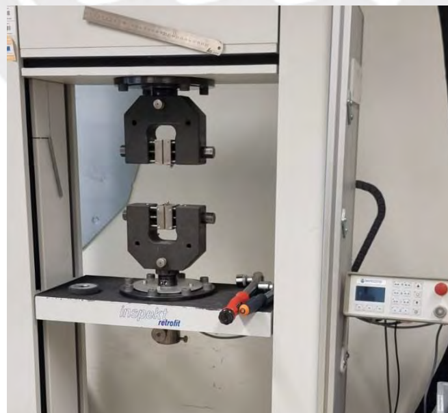
Figure 3.20. Tensile testing machine Hegewald & Peschke Inspekt Retrofit.
