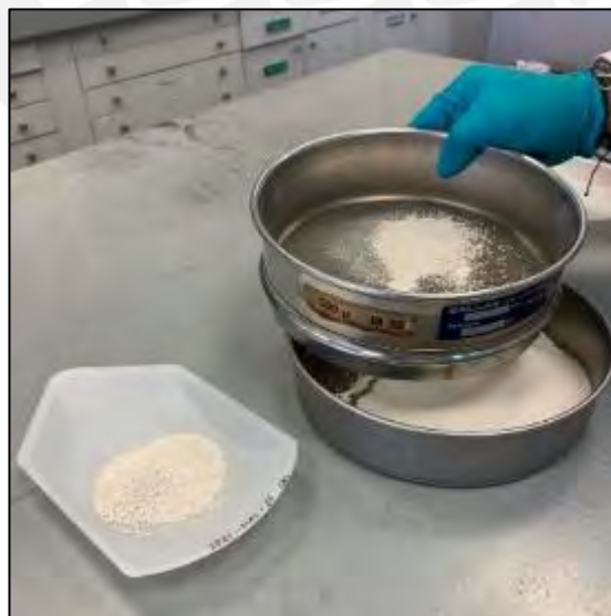
Figure 5. Dry sieving using a 500 \mu m sieve screen.
