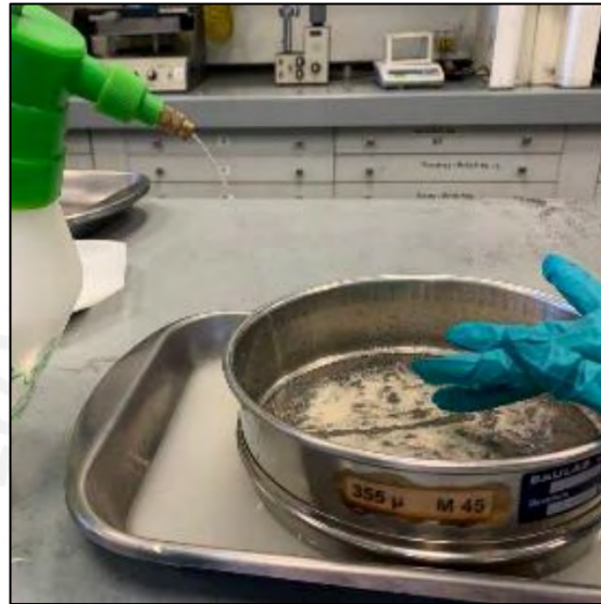
Figure 6. Wet sieving using wet sieving through a 355 \mu\text{m} aperture laboratory sieve.
