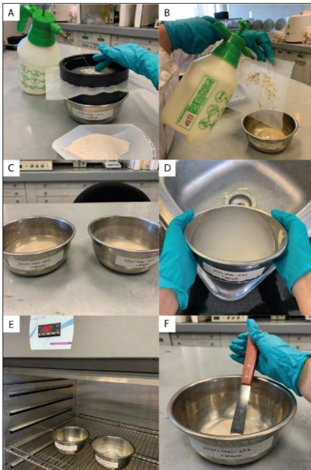
Figure 7. A: Sequential wet sieving of <355\ \mu\text{m} particulate material through disposable Nylon sieves ( 200\ \mu\text{m} , 100\ \mu\text{m} , 75\ \mu\text{m} , and 50\ \mu\text{m} apertures). B: Cleaning of the retained fraction on disposable sieves. C: Two bowls with coarse and fine (relative to the aperture of the used sieve) particulate material. D: Decantation for the elimination of very fine material (dust). E: Drying of the obtained granulometry fractions in a laboratory dryer at 50\ ^\circ\text{C} overnight. F: Dried sample ready for hydroseparation.
