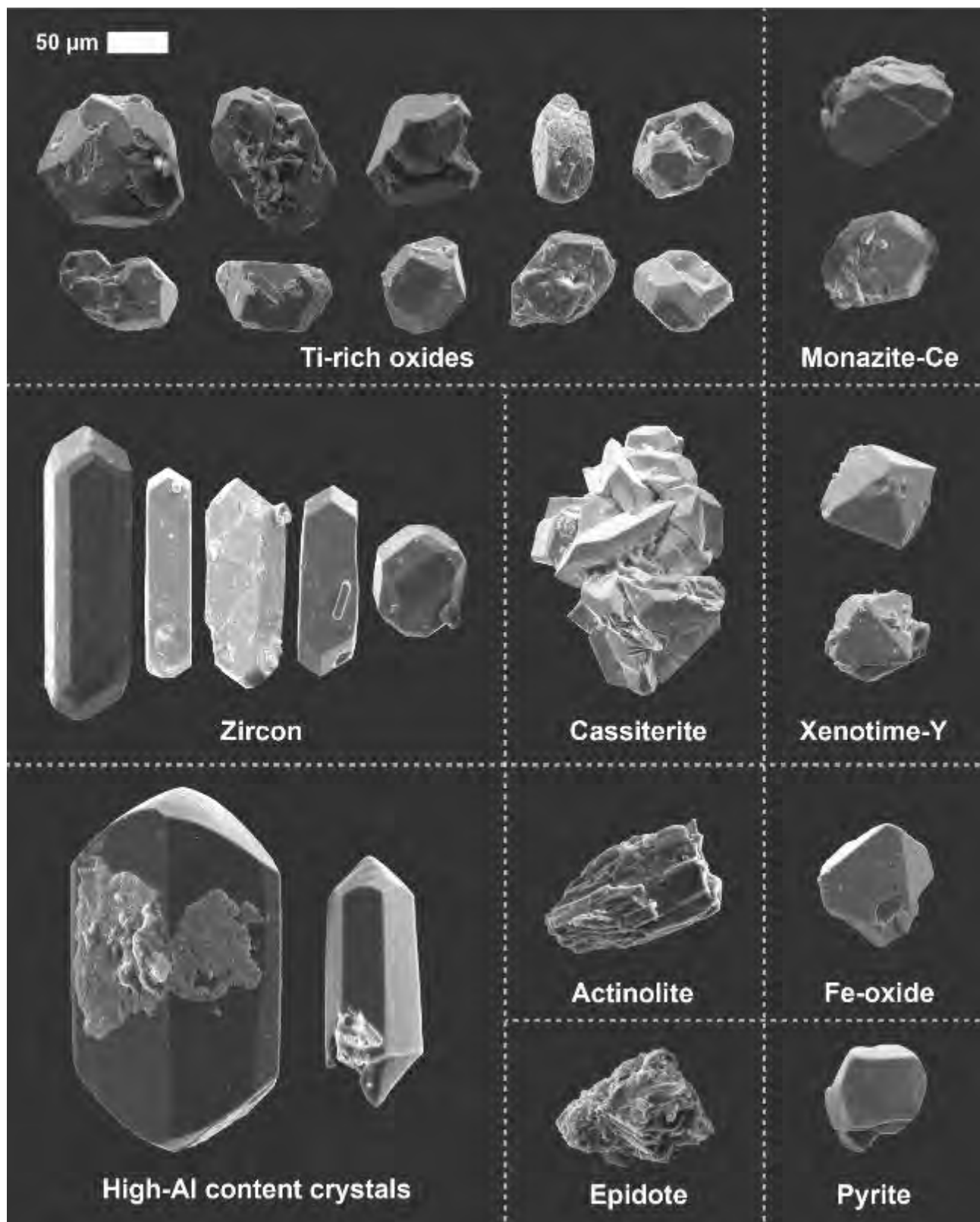
Figure 17. SEM-SE images of representative minerals found in heavy concentrates from sample 2021-MAC-08. See the main text for descriptions.
