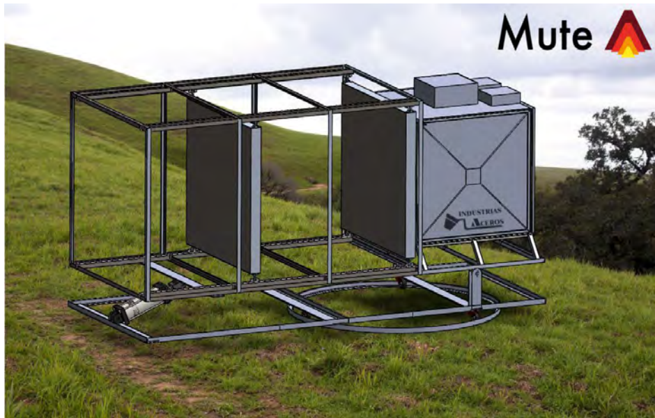
Figure 5.8: Structure of the Muon Telescope MuTe [10].
