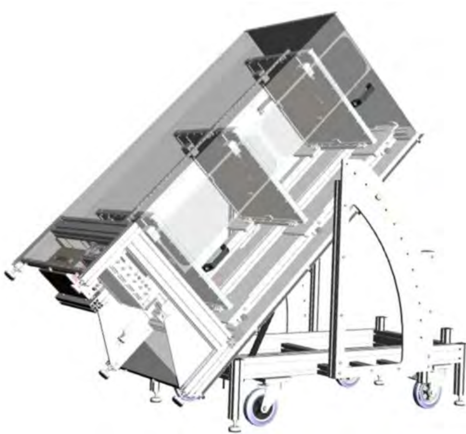
Figure 5.4: Schematic visualization of WatTo muon telescope based on Micromegas technology [79].
