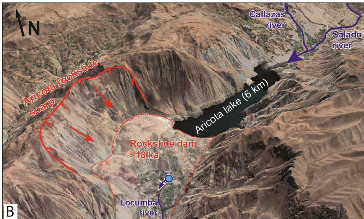
140 Figure 1: A) Study area location in the Central Western Andes and isohyets of annual precipitation; B) 3D 141 GoogleEarth view of the Aricota rockslide dam and its lake (modified from Delgado et al., 2020). The blue circle 142 locates a spring corresponding to the main seepage of the lake through the dam, feeding the lower Locumba 143 river. Overflow of water above the dam never occurred since the dam emplaced (Placzek et al., 2001).
