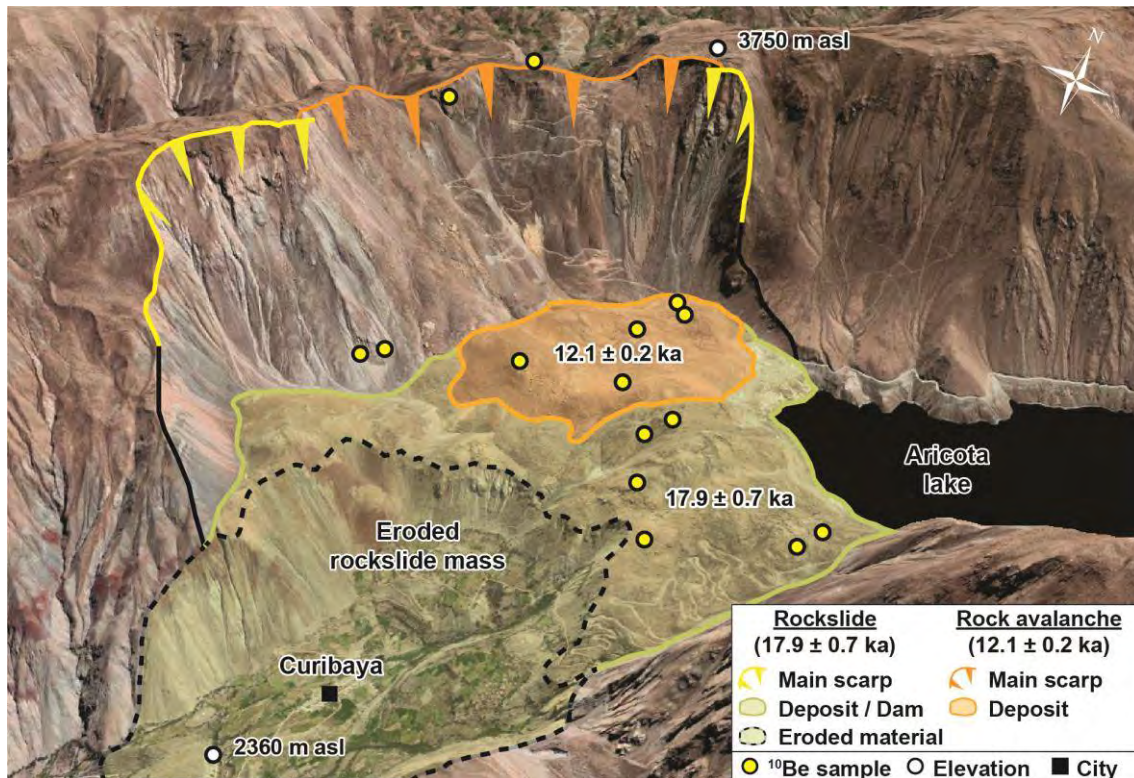
Figure 4. 3D Google Earth view of the Aricota rockslide (modified from Delgado et al., 2020). It is observed that the first event ( 17.9 \pm 0.7 ka) filled the valley and formed a big dam and the second event ( 12.1 \pm 0.2 ka) was deposited on top of the first event.
