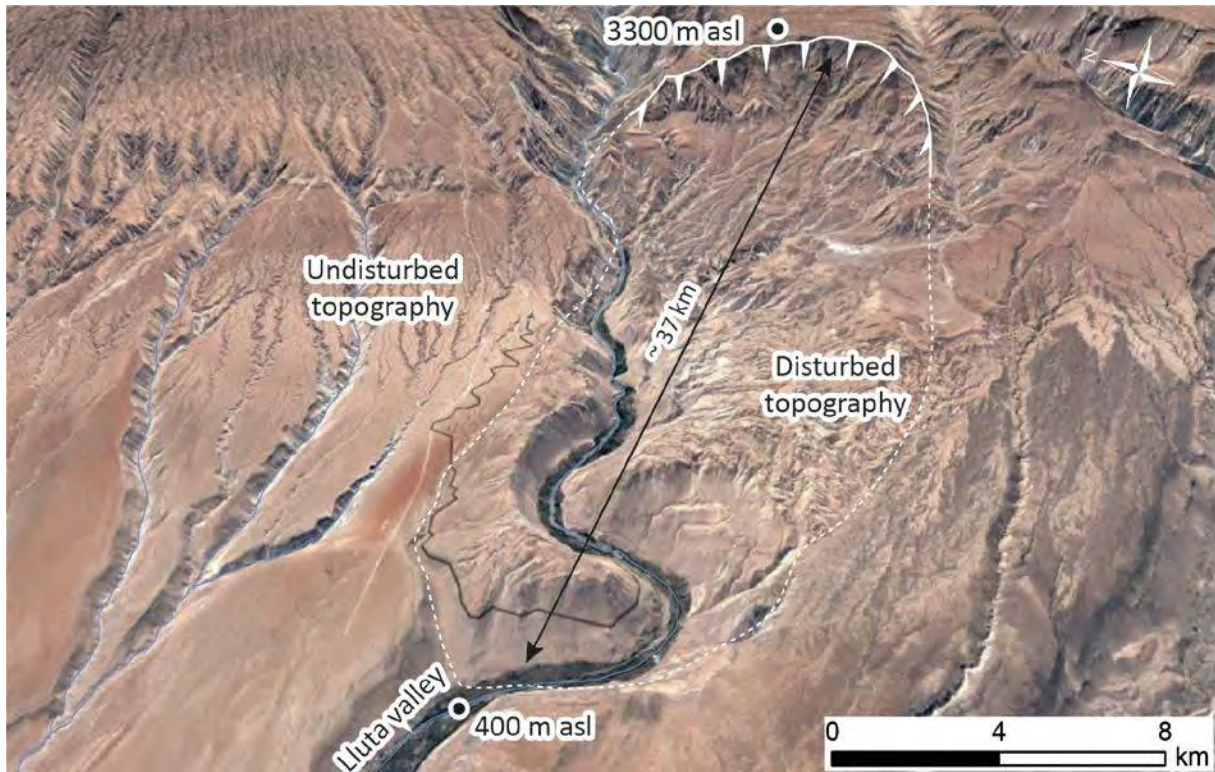
Figure 19. 3D view of the Lluta landslide, the 37 km long landslide mass disturbed the topography which was probably like the relief of the right flank of the Lluta valley.
