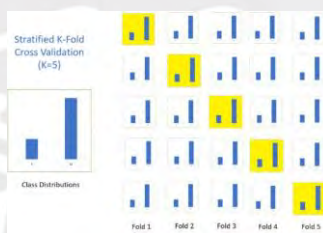
Figure 3.2: Stratified K-Fold Cross Validation ( Improve Your Model Performance using Cross Validation , n.d.)
