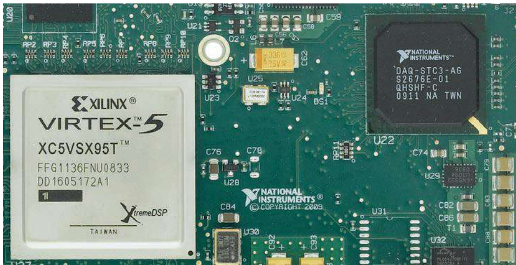
Figure 2. NI ASIC technology and Xilinx FPGAs provide a high-performance platform for flexible, user-customizable instrumentation.
