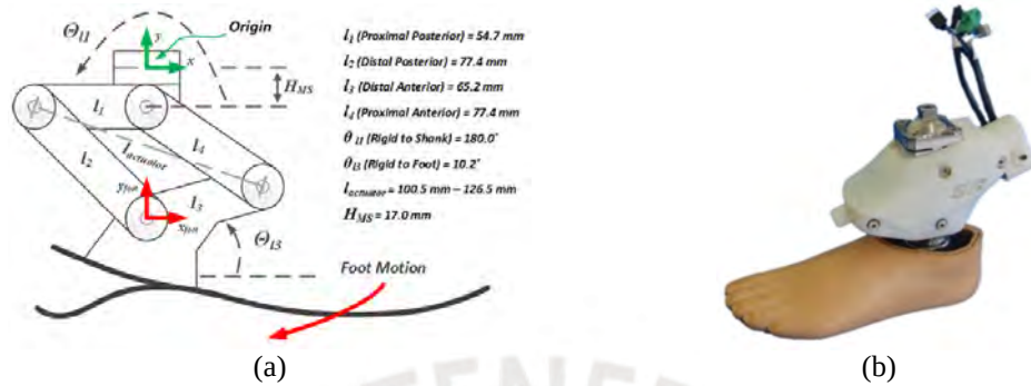
Fig. C6. Prótesis de University of Massachusetts Amherst: (a) mecanismo, (b) prototipo [Kennedy, 2016].
