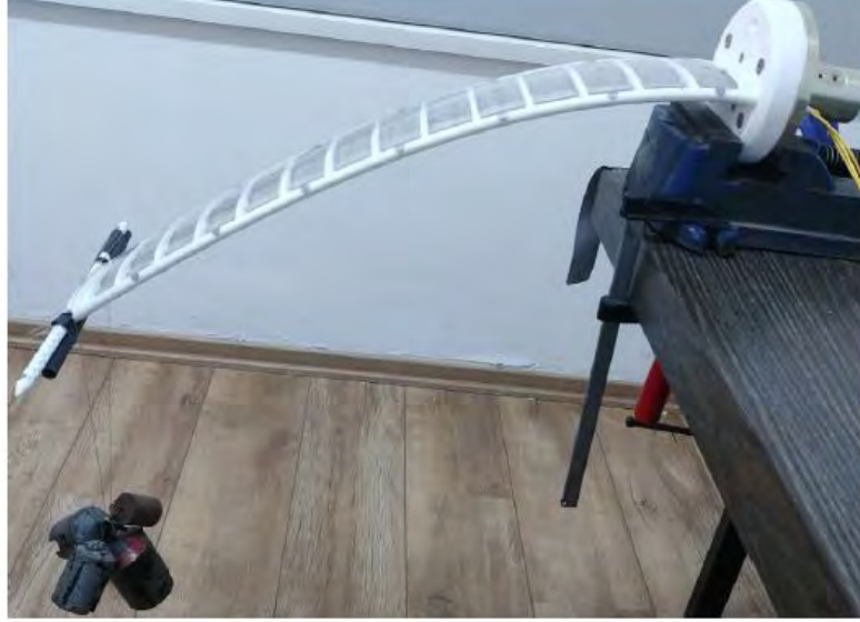
Figura 2.4: Structural testing on Pazy wing. Adapted from Riso y Cesnik (2023).
