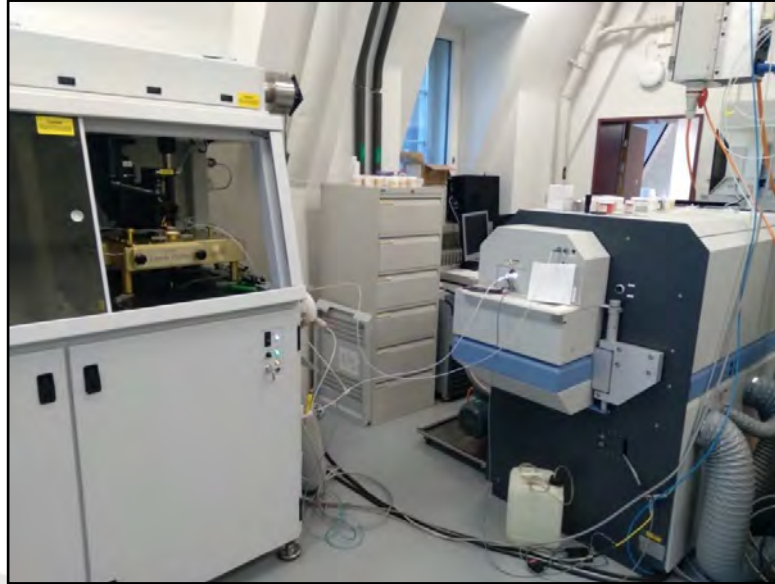
Figure 6. Thermo Scientific Element XR device with Laurin Technic S-155 ablation plate at ETH Zurich (Switzerland)
