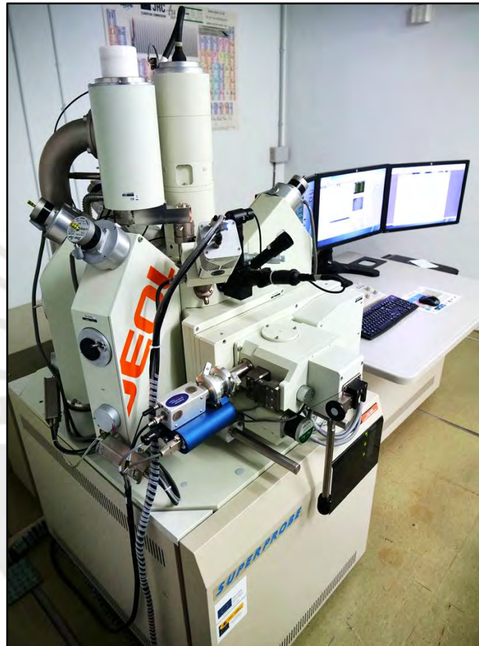
Figure 5. Electron microprobe equipment available at the Scientific and Technological Centers of the University of Barcelona, Spain
