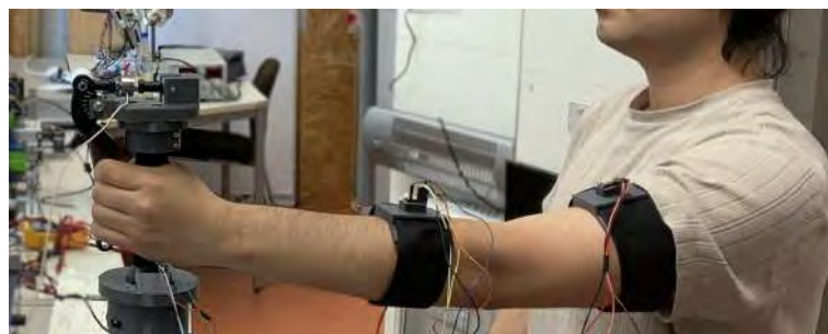
Figure 6.15.: Position of MPUs on the hand-arm-system: hand attached to the measurement device in a grip action (left) and test subject (right)
