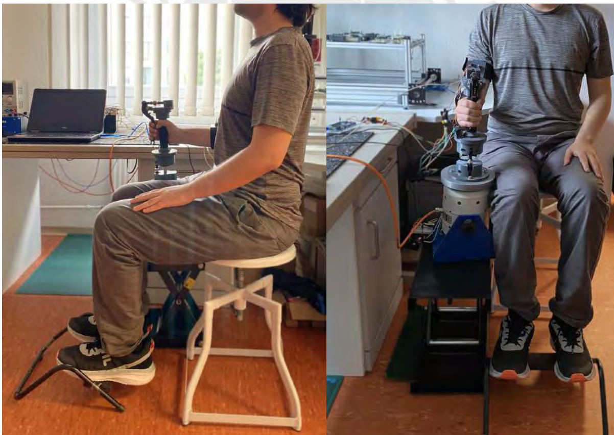
(a) Lifting platform for shaker positioning (bottom-behind), (b) shaker with measurement device (left-middle) footrest for 90° posture (bottom) and test subject and lifting platform (left-bottom) executing a grip action (middle-behind)
