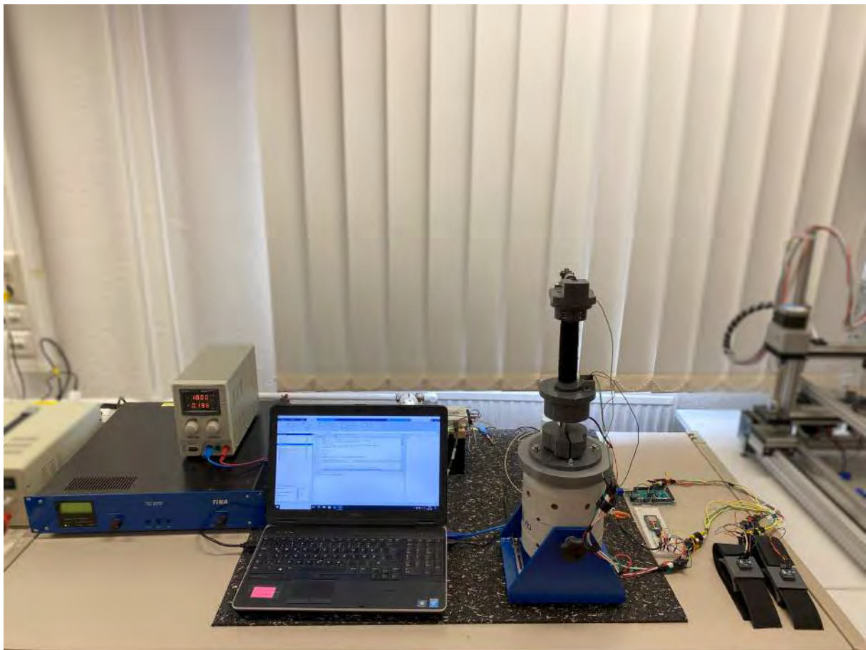
Figure 6.12.: Final measurement setup for experimental characterization: shaker amplifier and power source(left); computer and shaker with measurement device (mid front); force amplifier and DAQ (mid behind); IMUs with micro-controllers(right)
