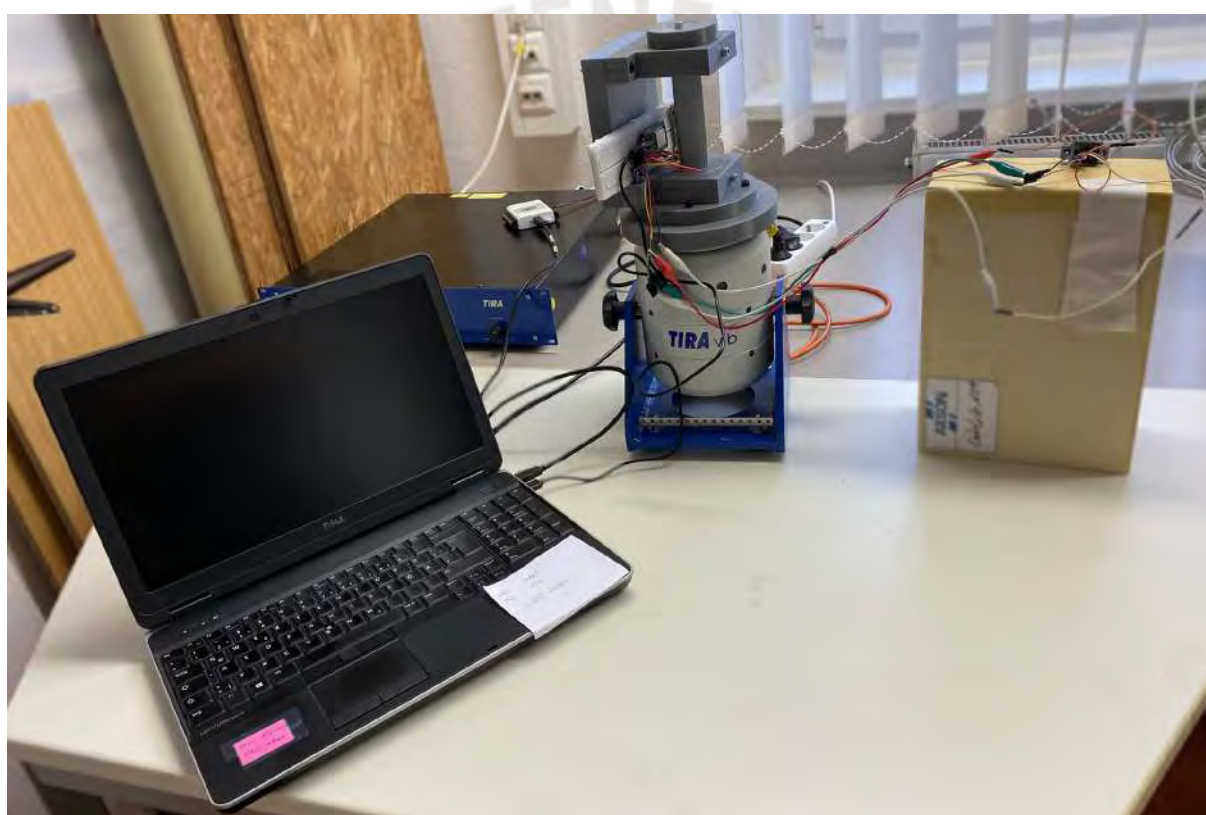
Figure 6.4.: First approach of measurement setup: shaker amplifier and DAQ (left behind), computer (left front), shaker with simplified device prototype and micro-controller with IMU (middle behind) and IMU (right)
