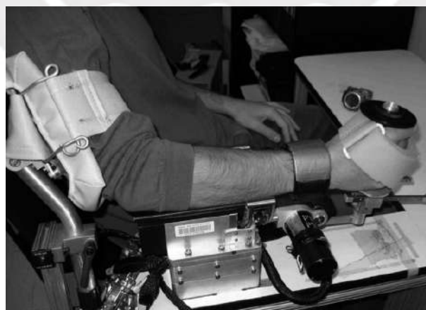
Figure 3.8.: ES for the determination of wrist stiffness in a relaxed state Formica et al. (2012)
