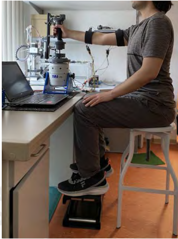
Figure 7.2.: Experimental setup with the test subject with a posture of 180^\circ between the forearm and upper-arm: lifting platform (bottom), measurement device with shaker (middle-left) and test subject (right)
