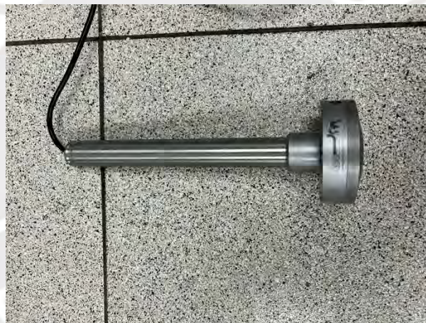
Figura 3.5 Celda de carga sumergible 10kN GDS
