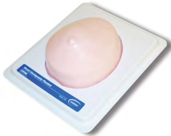
Figure 3.2: Calibrated breast phantom used for experiments.
