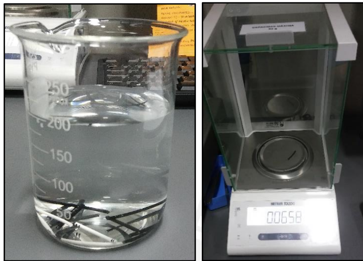
Figure 19. Imaging of the water absorption analysis (filaments water immersion and filaments weight)
