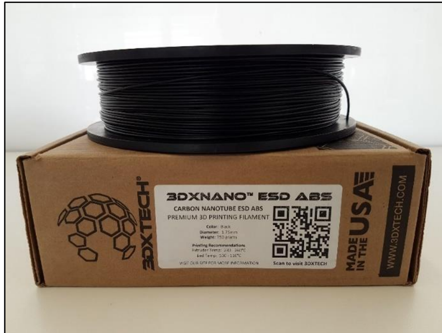
Figure 14. ABS/CNT FDM filament (3DXNano™ ESD ABS)
