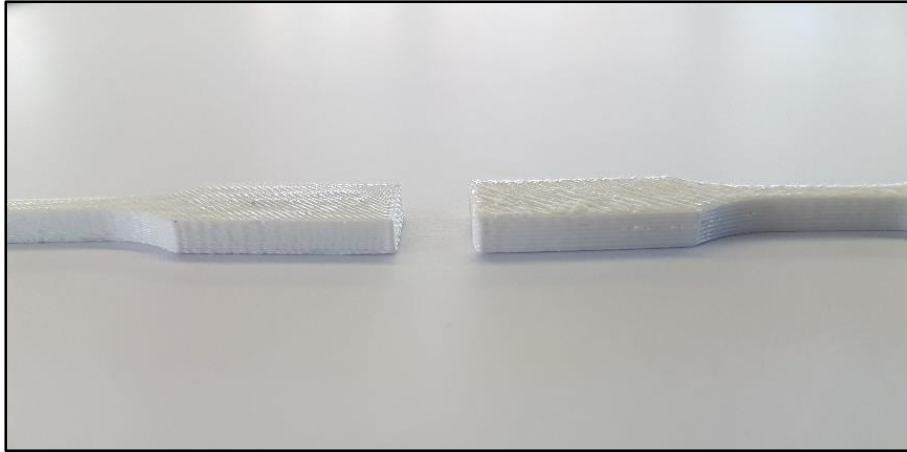
Figure 13. FDM pure ABS tensile specimens
