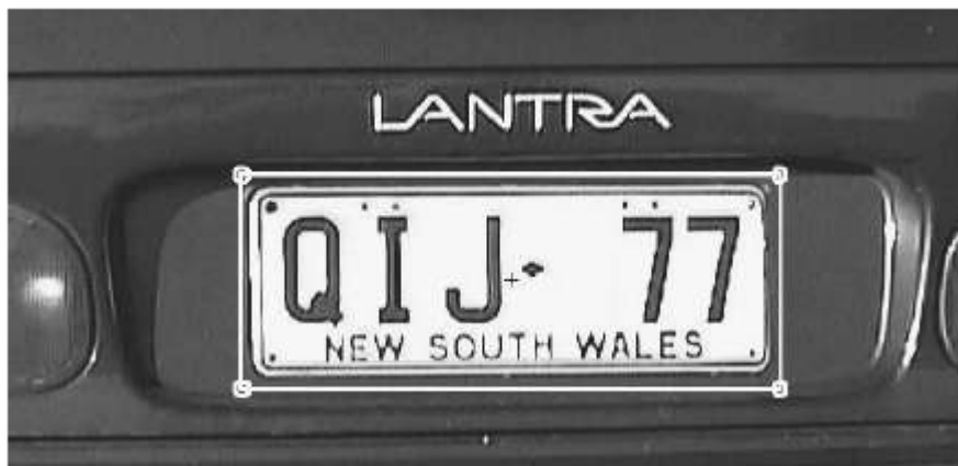
Figure 2.12: Region of interest (ROI). Car license plate with a defined ROI [16].
