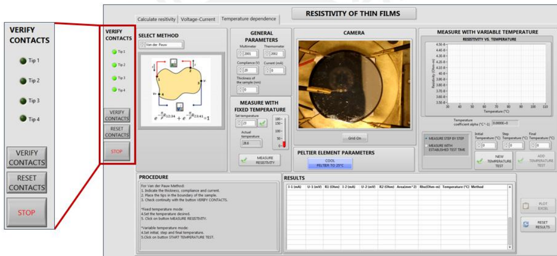
Figure 3.22: GUI of the measuring system developed with LabVIEW. Verify contacts area.
