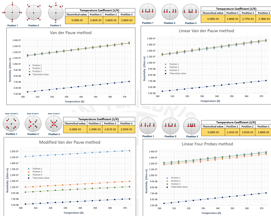
Figure 4.14: Resistivity dependence on the temperature of a tungsten thin film sample with 300 nm thickness. The theoretical temperature coefficient of the tungsten is shown in the tables.
