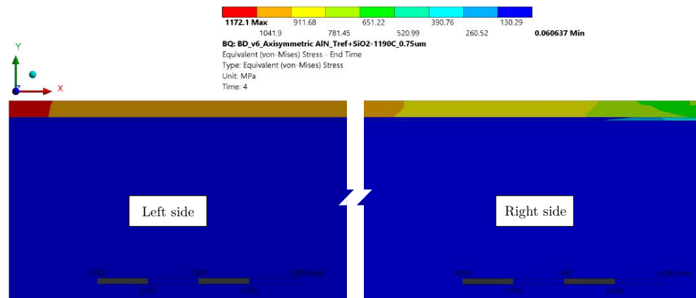
Figure 3.26.: Distribution of equivalent stresses (von Mises) in MPa generated in the AIN axisymmetric model from the left to the right side of the model.
