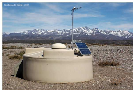
Figure 4.5: Cherenkov Tank of Pierre Auger Observatory (Auger-Collaboration, 2015).
