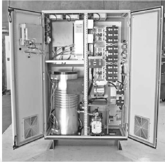
Figure 1.12: 125 kW energy storage flywheel in cabinet for UPS application and ride-through service by author [BZW12].
