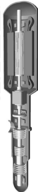
Figure 1.13: Turbo generator for a nuclear power plant. The specifications are: 6 MW, 15000 rpm, vertical rotor axis, 4 radial bearings, 2 axial bearings, length of turbine 3.5 m and mass of turbine 1000 kg. By author [SGLY06].
