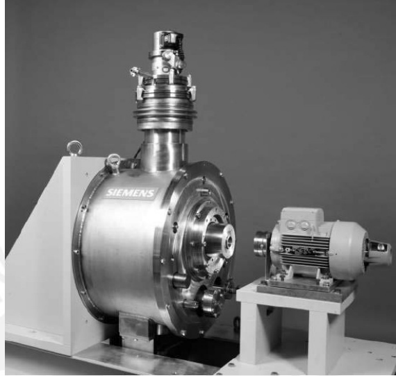
Figure 1.14: Superconductive bearing. The specifications are: bearing capacity 500 kg and maximum speed 4500 rpm. By author [KNN06].
