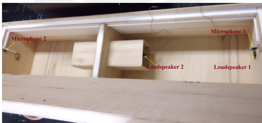
Figure 4.6: Interior of the ANC system prototype
