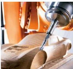
Direct execution of all standard G and M commands for tool handling and HSC (High-Speed Cutting).
