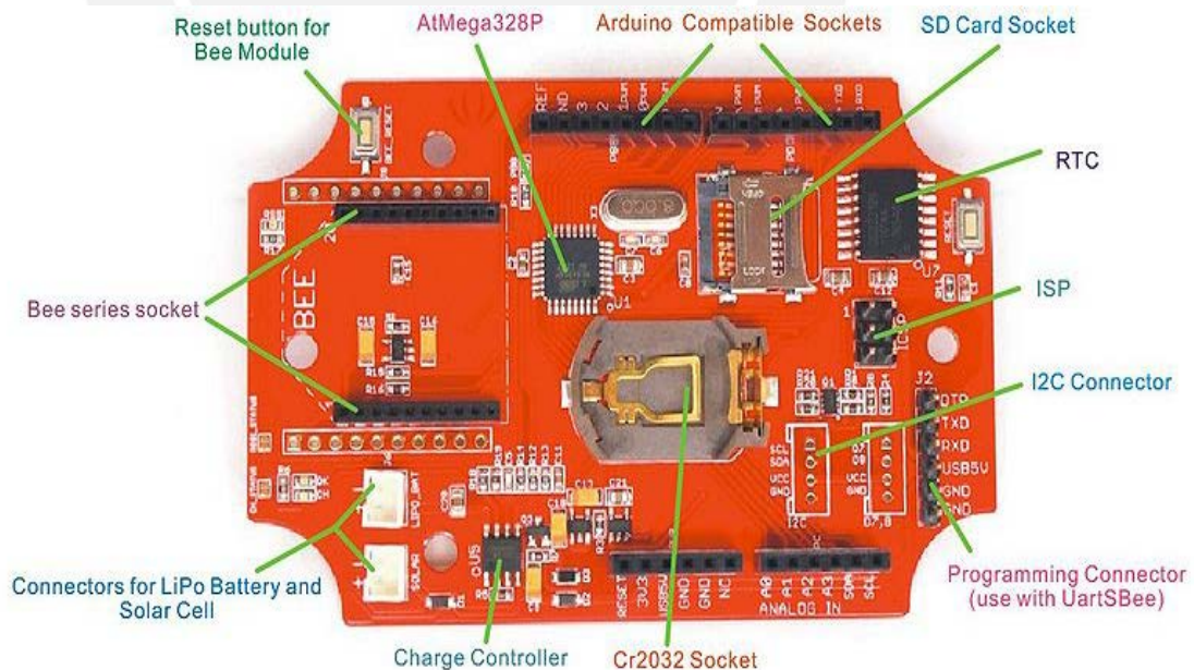
Fig. 1.1 Partes de la mota Seeeduino Stalker V2.3 [40]
