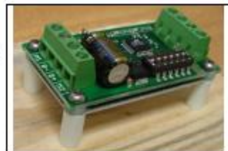
Figure 2.3: Mounted to a wood frame using standoffs
