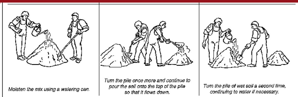
Figura 2.3 Cribado manual (Guillaud et al. 1995)
