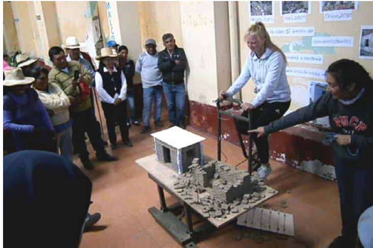
Figure 6. Dynamic test with the portable shaking table.
