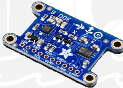
Figura 3.2. Adafruit 9-DOF IMU Breakout.
