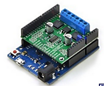
Pololu dual MC33926 motor driver shield, assembled and connected to an Arduino Leonardo.
