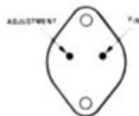
Figure 1. (TO-3) Metal Can Package Case is Output Bottom View See Package Number NDS0002A
