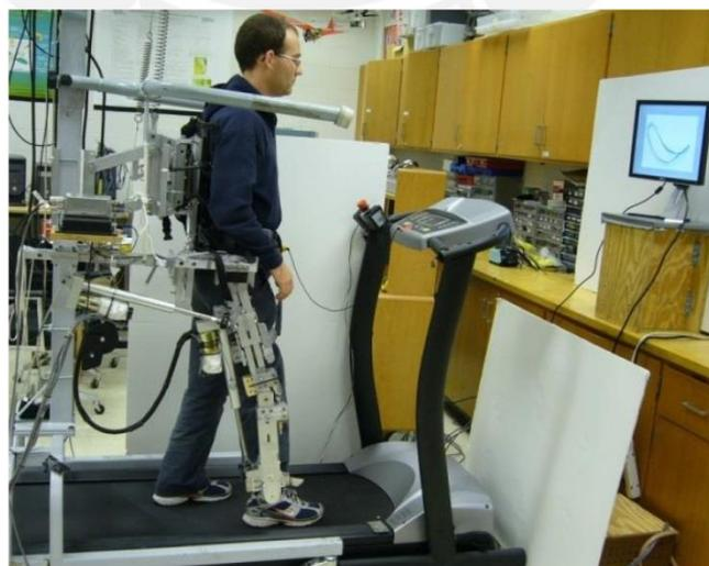
Figura 1.21: Active Leg Exoskeleton (ALEX) [SAI, 2007]
