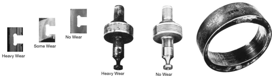
Figure 1. Typical Examples of Wear Due to Contamination
