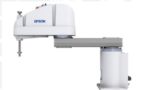
Figura 1.5: Robot S.C.A.R.A. [6]
