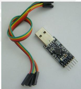
Figura 3.5: Conversor USB a Serial TTL
