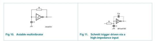
If a Schmitt trigger is driven via a high-impedance (R > 1 k $\Omega$ ), then it is necessary to incorporate a capacitor C with a value of  $\frac{c}{C_P} > \frac{V_{DD} - V_{SS}}{V_H}$ ; otherwise oscillation can occur on the edges of a pulse.
