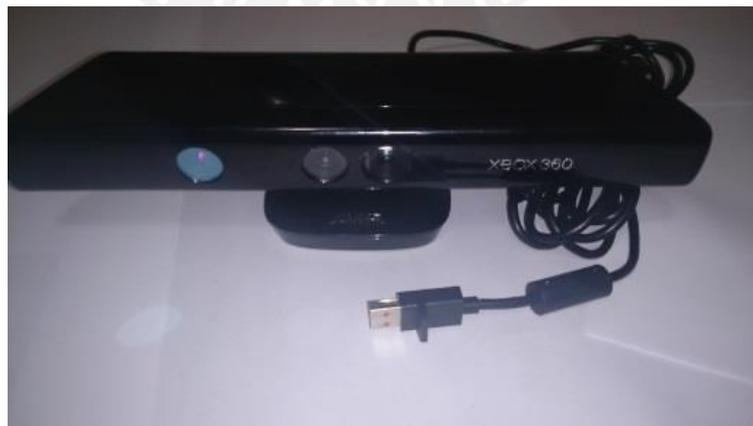
Figura 2.1 Sensor Kinect.
