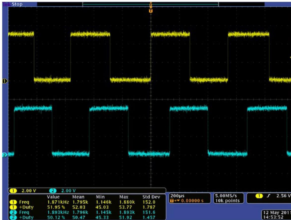
Encoder A and B outputs for 25D mm HP metal gearmotor with 48 CPR encoder (motor running at 6 V).
