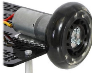
A 25D mm gearmotor connected to a scooter wheel by the 4 mm scooter wheel adapter.
