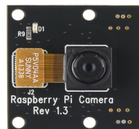
Figura 3.15. Raspberry Pi Camera – NOIR.[22]
