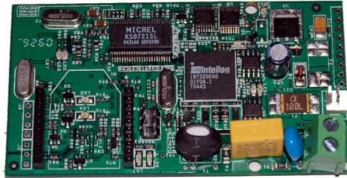
A LinkSprite high speed PLC-UART
