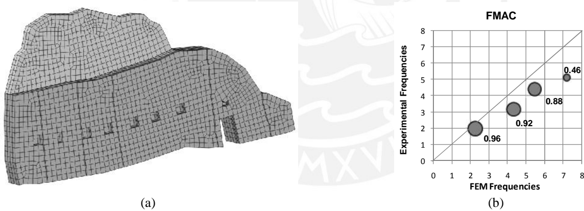
Fig. 6- Model1: (a) FE numerical model; and (b) comparison between numerical and experimental results
