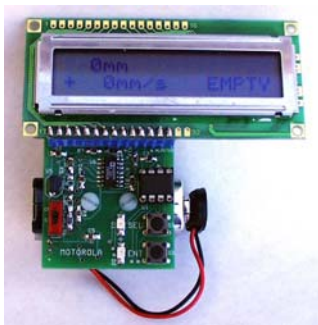
Figure 1. Water Level Reference Design Featuring a Pressure Sensor
