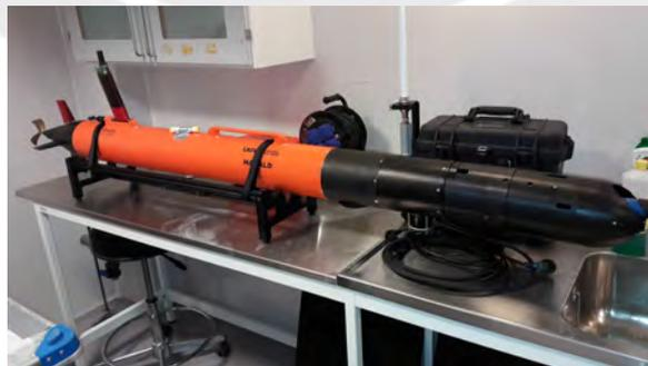
Figura 1.4 Robot submarino LAUV-Harald
