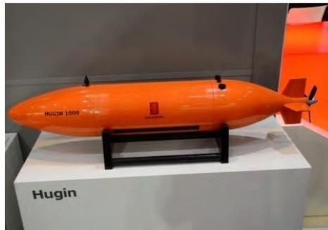
Figura 1.5 Robot submarino AUV Hugin
