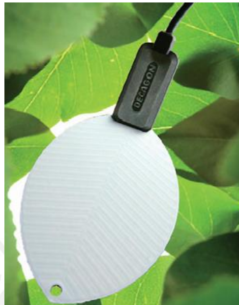
FIGURA 1-6 Leaf Wetness Sensor de la empresa Decagon Devices Inc.
